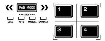
**HOT CUE mode**: Pads 1-4 trigger Serato DJ Pro Cue points, and if no Cue point is present on that slot/pad, pressing that pad will set a Cue point. Holding down the **PAD MODE** button while pressing a pad will delete the Cue point from the respective pad/slot.
