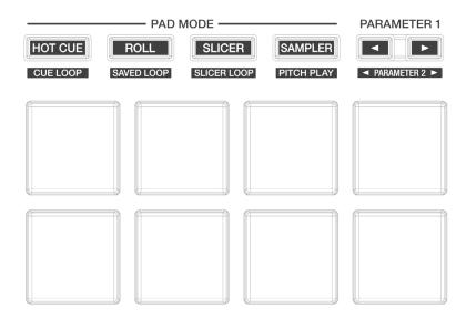
**CUE LOOP mode**: Hold SHIFT while pressing the HOT CUE mode button to enter CUE LOOP mode. Pads 1-8 trigger Serato DJ Pro Cue points but also triggers an autoloop of variable sizes. If the selected slot has no Cue point present, one will be set. Holding SHIFT while pressing a pad will retrigger that Cue Loop. Use the Parameter left & right buttons to increase or decrease the loop size.
