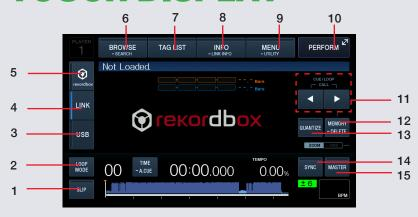
To enter the performance mode as shown in the image below, press the perform button on the XDJ-1000 Touch Display. You can also show Auto-Loop options by pressing the button.
