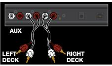
Connect the OUTPUTS of the SL 3 to line inputs on your mixer. Connect the AUX output to an additional line input or AUX input on your mixer to output the sample player. **SEE "SAMPLE PLAYER" ON PAGE 18.**
