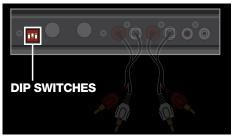
Set each input to the correct input level using the dip switches. Set the switches UP for Phono (turntables) or DOWN for Line (CD players).
