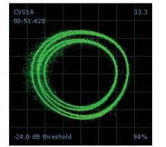
**RECORD BURN** - This section of the control vinyl has been worn. Swap sides or use the track start offset.
