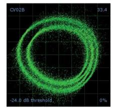
**UNEARTHED** - Very susceptible to interference. Attach the turntable's ground wire.
