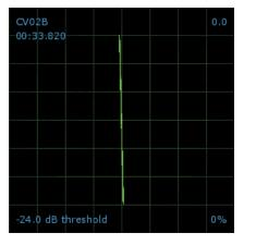
**LEFT CHANNEL MISSING** - The signal from the needle is not reaching the SL 3. Check the cable and cartridge connections.
