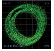
**USING PIGGYBACK CABLES** - Picking up huge amounts of noise, barely tracking. Connect your turntables directly to the hardware.
