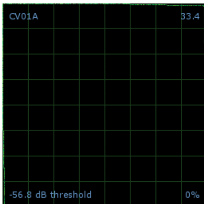
CD PLAYER INTO PHONO INPUT - Scratch Live is set to receive phono level input. Set to the correct value in the setup menu.
