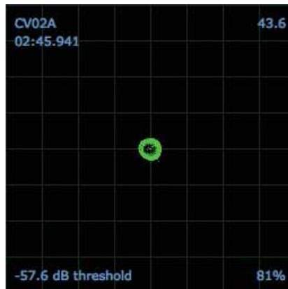
PHONO INTO LINE INPUT - Scratch Live is set to receive line level input. Set to the correct value in the setup menu.
